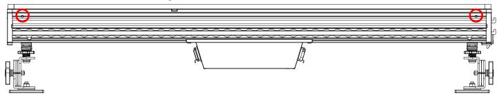
2. Align the thumbscrews of the Glare Shield with the mounting screw holes and insert them.
