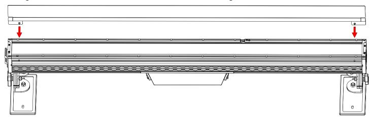
3. Tighten the two thumbscrews to secure Glare Shield. Thumbscrews can also be tightened with a Phillips screw driver.
