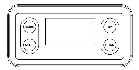
This fixture includes a display lock feature which automatically shuts off the display screen after a certain period of inactivity. This feature is OFF by default, which means that the display will always remain on regardless of inactivity, but can be configured to kick in after up to 10 minutes of inactivity.
