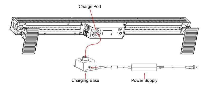
**Disconnect the unit from the charger once the battery is fully charged.** Doing so reduces the risk of overcharging the battery, which can shorten the service life of the battery.
