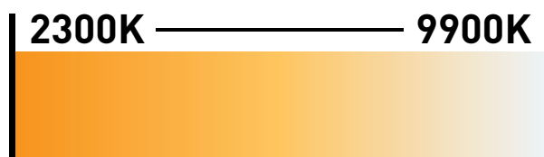
LINEAR COLOR TEMPERATURE CONTROL (TUNABLE WHITE)
