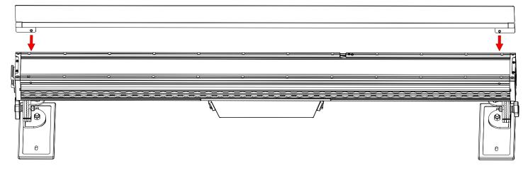
3. Tighten the two thumbscrews to secure Glare Shield. Thumbscrews can also be tightened with a Phillips screw driver.
