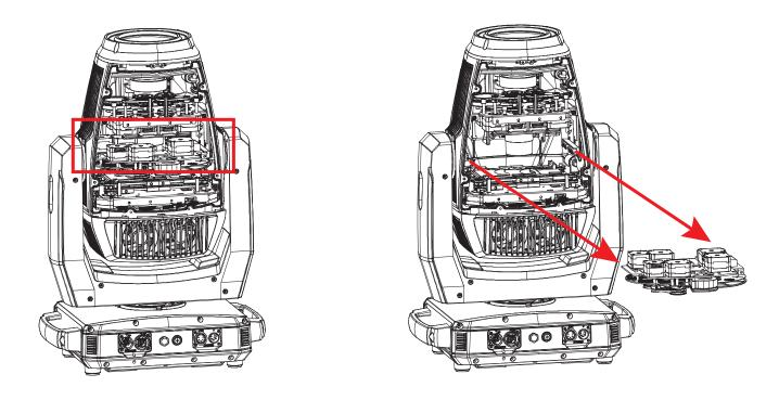
4. Pull the gobo holder away from the gobo wheel, then gently slide it outwards. Use a pair of needle nose pliers to carefully remove the retainer spring from the gobo holder. The gobo can now be removed from the gobo holder, and replaced with a new gobo. Reassemble by reversing these steps.
