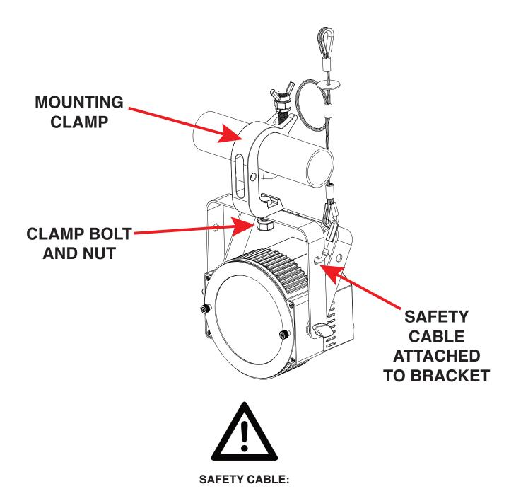
ALWAYS ATTACH A SAFETY CABLE WHENEVER INSTALLING THIS FIXTURE IN A SUSPENDED ENVIRONMENT TO ENSURE THAT THE FIXTURE WILL NOT FALL IF THE CLAMP FAILS.
