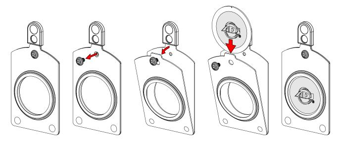
On the barrel, loosen knobs to slide plate forward, revealing slot. Insert holder into slot, front facing forward, slide plate back, tighten knobs.
