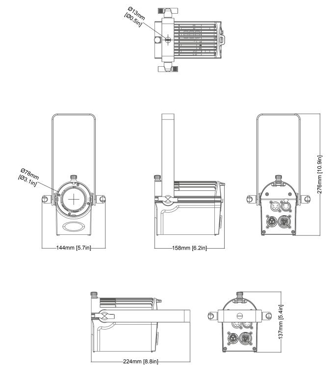
Note: Height may depend on thumb screw tightness. Overall height when fully tightened is 137mm (5.4in) as shown below. Overall height with thumb screw loosened is 140mm (5.5in).
