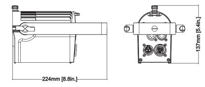
Note: Height may depend on thumb screw tightness. Overall height when fully tightened is 137mm (5.4in) as shown below. Overall height with thumb screw loosened is 140mm (5.5in).
