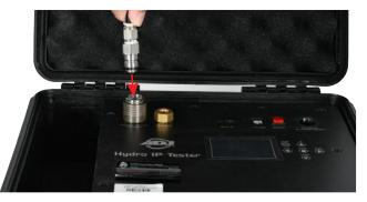
1. Connect the air hose quick-connect fitting to the Hydro IP Tester.
