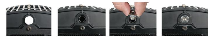
3. If the fixture has a second pressure relief valve, remove and replace it with an M12x1.5 Hex Socket Cap Head A4-70 Stainless Steel Bolt/Washer (included), and tighten using a 6mm Hex Wrench. **NOTE: Make sure the bolt has its O-ring for a proper seal.**
