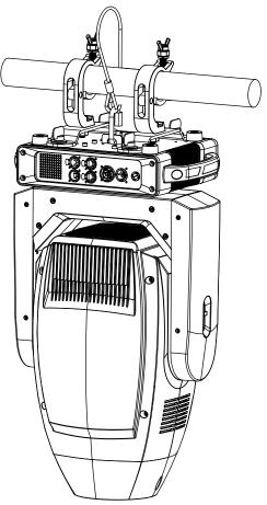
When installing the unit, the trussing or area of installation must be able to hold 10 times the weight without any deformation. When installing the unit must be secured with a secondary safety attachment, e.g. and appropriate safety cable. Never stand directly below the unit when mounting, removing, or servicing the unit.
