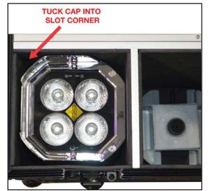
4. Place an ADJ Mirage Q IP device in any of the device slots in the flight case. Up to 6 devices can be accommodated. The charge indicator located beside the power ports will illuminate to indicate that your device is charging. It is strongly recommended to leave the case lid open during charging.
