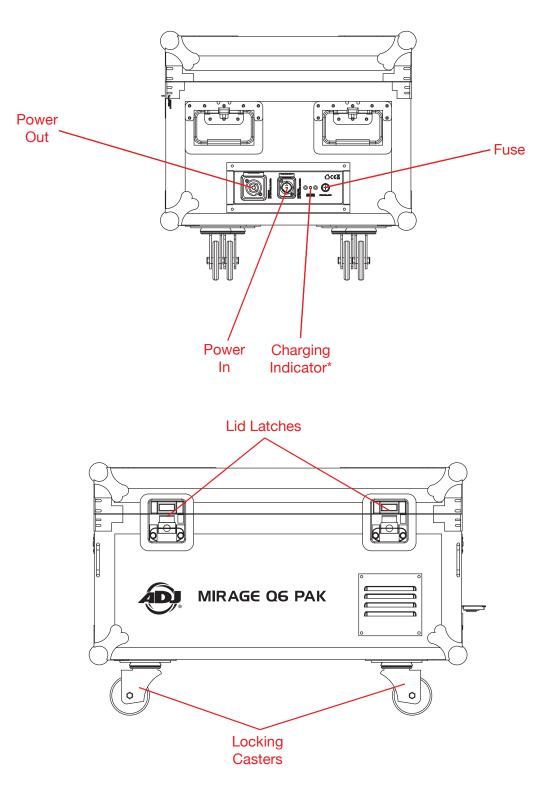
\*Note: Charge indicator is red when charging, and green when complete. Charge indicator on the case displays charge status of the entire six-unit set. For individual charge status, please refer to the charge indicator on each individual unit.
