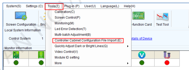
Figure 5-4 Importing controller cabinet configuration files
