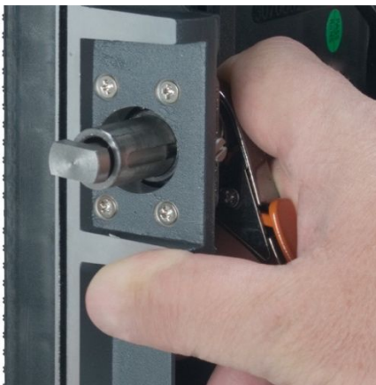
3. Turn the panel connector lever down to lock
